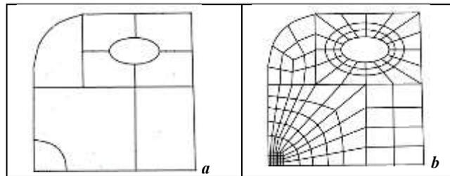
**Figure 2. The studied area breaks into a set of elementary areas and formation of discrete model of a difficult configuration**
