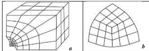
*Figure 3. A parallelepiped with ellipsoidal dredging in top and finite element representation of an ellipsoidal triangle*
